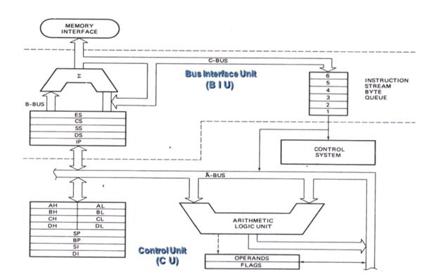
In order to speed-up the processing, the 8086 architecture is divided into two independent functional units; the Bus Interface unit (BIU) and the execution unit (EU).
