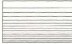
Fig. 6-11 Crowding at bottom caused by nonlinear vertical scanning.
