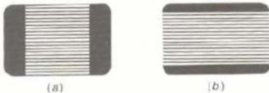
Fig. 6-7 Incorrect aspect ratio in raster. Black areas show areas of the screen not covered by the scanning lines. (a) Insufficient width. Too much black area at left and right sides. (b) Insufficient height. Too much black area at top and bottom.
