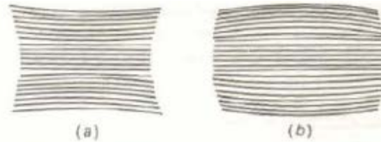
Fig. 6-8 (a) Pincushion effect in raster. (b) Barrel distortion.
