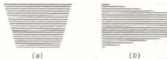
Fig. 6-9 Trapezoidal raster. (a) Keystoned sides caused by unsymmetric horizontal deflection. (b) Keystoning at top and bottom caused by unsymmetric vertical deflection.
