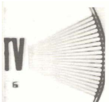
Fig. 6-12 Example of faulty interlacing. The line divisions in horizontal wedges of test pattern are interwoven in a moiré effect.
