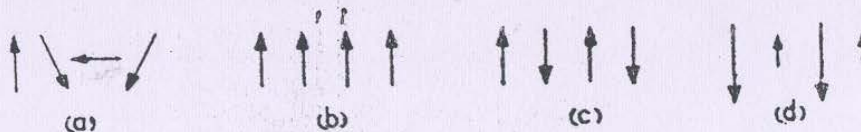
Fig. 6.3. Paramagnetic, ferromagnetic, anti-ferromagnetic and ferrimagnetic arrangement of spins.
