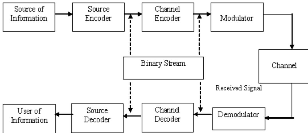
*Fig 1.: Block Diagram of a Digital Communication System*
