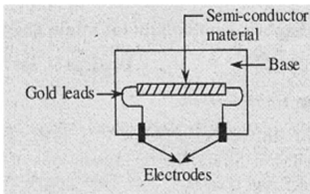
fig.9.a. Semiconductor Strain gauge
