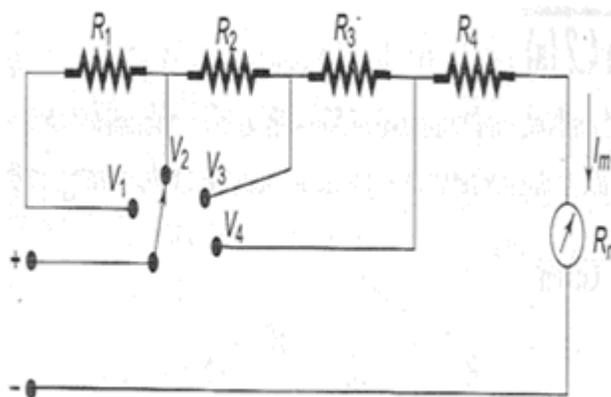
fig 4. a. (ii) Multiplier Connected in Series String
