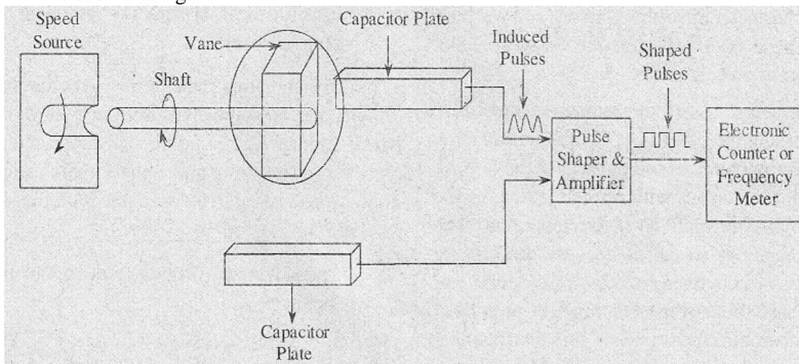
fig 8.b. Capacitive Transducer
