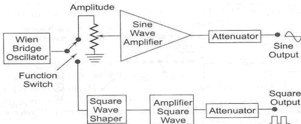
fig.6.a.(ii) AF sine & Square wave generator
