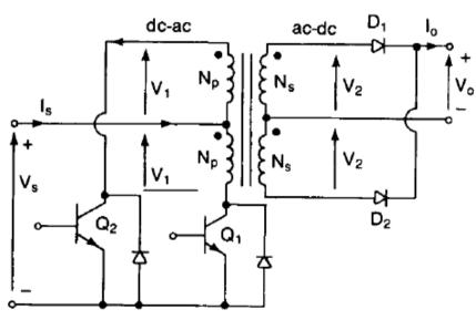
The average (or dc) output voltage of the push-pull circuit shown above is 24 V with<br/>the resistive load of 0.8 ohms. The on-state voltage drops of transistors and diodes are<br/>1.2 V and 0.7 V respectively. The turns ratio of the transformer is 0.25. Determine<br/>(i) Average input current(ii) Efficiency(iii) Average transistor current(iv) Peak transistor current(2+3+2+3)
